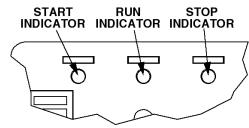
STOP indicator illuminated = STOP contact closed RUN indicator illuminated = RUN contact closed START indicator illuminated = START contact closed
